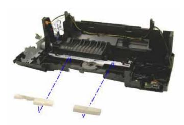
Because the chassis and platen (or other parts) have to be removed to replace the ink absorber, head-to-paper distance may be misaligned.
