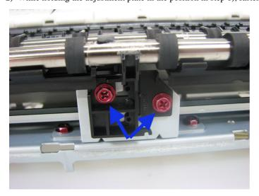
3) After assembly of the platen unit, be sure to perform the service test print, and confirm that no strange noise or faulty printing (uneven printing or contact of the print head to the paper) occurs.
