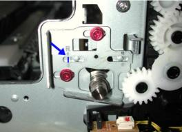
2) Remove the red screws from the adjusting plate.
