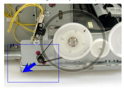
Note: The red screws securing the paper feed motor may be loosened only at replacement of the paper feed motor unit. DO NOT loosen them in other cases.
