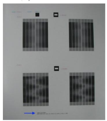
Confirm that "OK" is printed at the bottom of the paper (the blue arrow-indicated area in the photo above). If "NG" is printed, perform steps 3) to 5) again.
