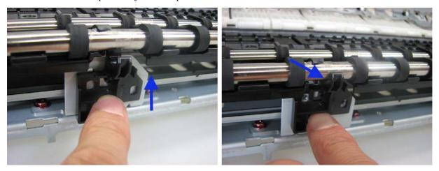
2) While holding the adjustment plate in the position in step 1), fasten the red screws.
