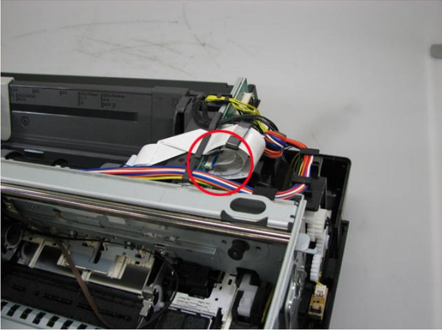
8) Slide the carriage unit to the center (the ink tank replacement position). While slightly pulling the front stay toward you, remove the carriage unit.
