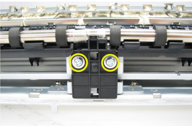
7) Remove the timing slit disk and the eject encoder holder. (1 screw)
