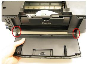
7) Remove the panel cover unit (1 screw).
