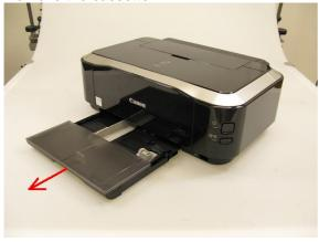
2) Remove the paper support unit and the access cover.
